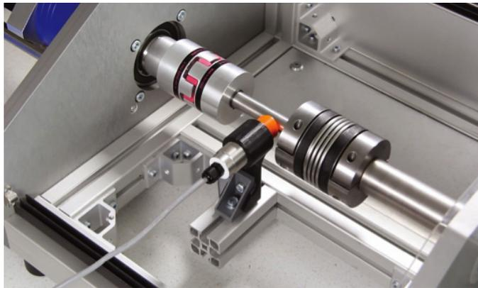
*TAM's active torque sensor kit is designed for an easy installation (top) When in situ it is a true non-contact sensor (above)*
